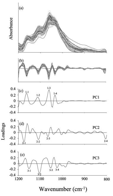
Fig. 2. (a) FT-IR spectra; (b) secondary derivative peaks; (c) score loadings of PC1. The bands labeled 1-1 to 1-4 correspond to wavenumbers near 1164, 1110, 1060 and 1033 cm<sup>-1</sup>. (d) Score loadings of PC2. The bands labeled 2-1 to 2-4 correspond to wavenumbers near 1170, 1110–1106, 1068–1064 and 806–802 cm<sup>-1</sup>. (e) Score loadings of PC3. The bands labeled 3-1 to 3-4 correspond to wavenumbers near 1152,1102, 1052 and 1025 cm<sup>-1</sup>.
