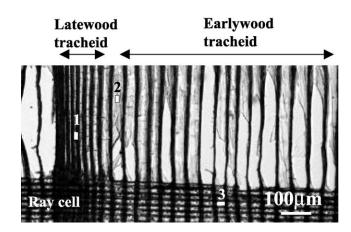
Fig. 1. A typical sample image of a wood section. The small white areas indicate the areas scanned by FT-IR Notes; 1. Latewood tracheid. 2. Earlywood tracheid. 3. Ray parenchyma cell.
